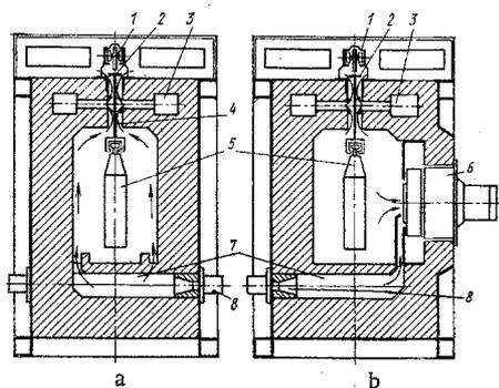
Fig. 5. Cross section of high-temperature (a) and low-temperature (b) overhead conveyor furnaces. 1) Overhead conveyor; 2) covered slots; 3) flue; 4) hanger; 5) forging; 6) device for recirculating combustion products; 7) combustion chamber; 8) burner.
