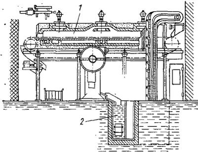
Fig. 3. Diagram of apparatus for heat treatment of forgings with utilization of forging heat. 1) Conveyor tempering furnace; 2) quenching tank.
