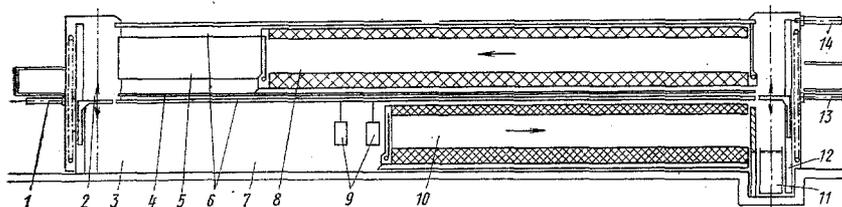
Fig. 4. Diagram of double-deck apparatus for heat treating forgings (furnaces with overhead conveyors). 1) Pusher; 2) elevator; 3) unloading station; 4) working area; 5) cooling tunnel; 6) overhead conveyor; 7) loading station; 8) tempering furnace; 9) hangers with forgings; 10) quenching furnace; 11) quenching tank; 12) elevator; 13) unloading device; 14) pusher.
