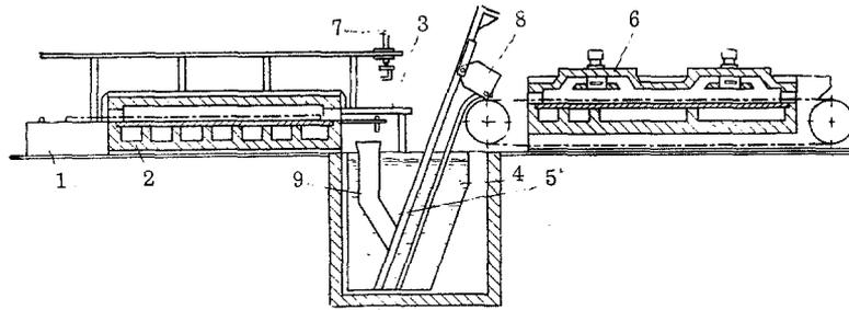
Fig. 2. Diagram of apparatus for quenching and tempering of forgings.
