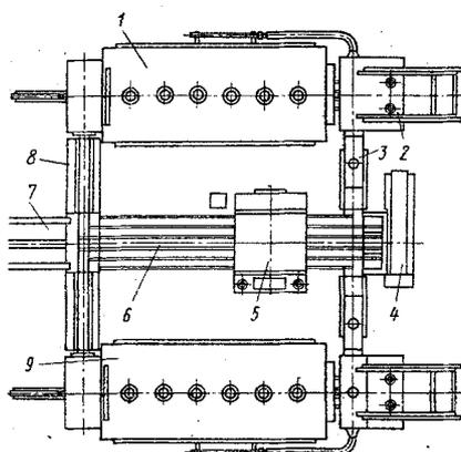
Fig. 1. Apparatus for heat treating forged turbine blades. 1) Pusher quenching furnace; 2) quenching device; 3) air spray; 4) belt conveyor; 5) washer; 6) intermediate conveying device; 7) loading station; 8) transporting device to feed forgings to furnace; 9) pusher tempering furnace.
